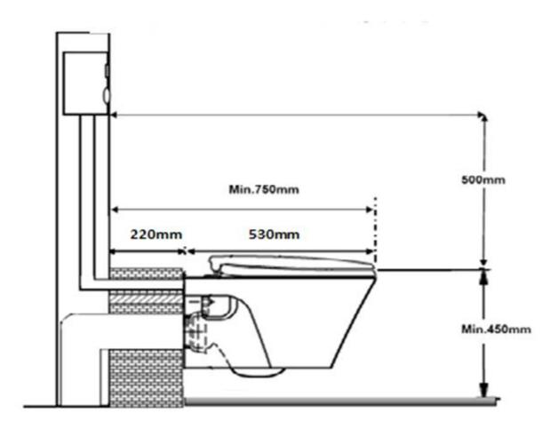
To meet the requirement of BCA Accessibility Code 2013 for Acessible indivdual washroom an extension low wall have to be built to meet the length of 750mm
